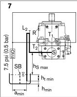
$h_{s max} = 31.50 \text{ in (800 mm)}, h_{t min} = 7.87 \text{ in (200 mm)}, h_{min} = 3.94 \text{ in (100 mm)}, SB = Silencer plate (baffle plate)$
