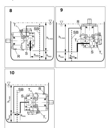
$h_{s max}$  = 31.50 in (800 mm),  $h_{t min}$  = 7.87 in (200 mm),  $h_{min}$  = 3.94 in (100 mm), SB = Silencer plate (baffle plate)
